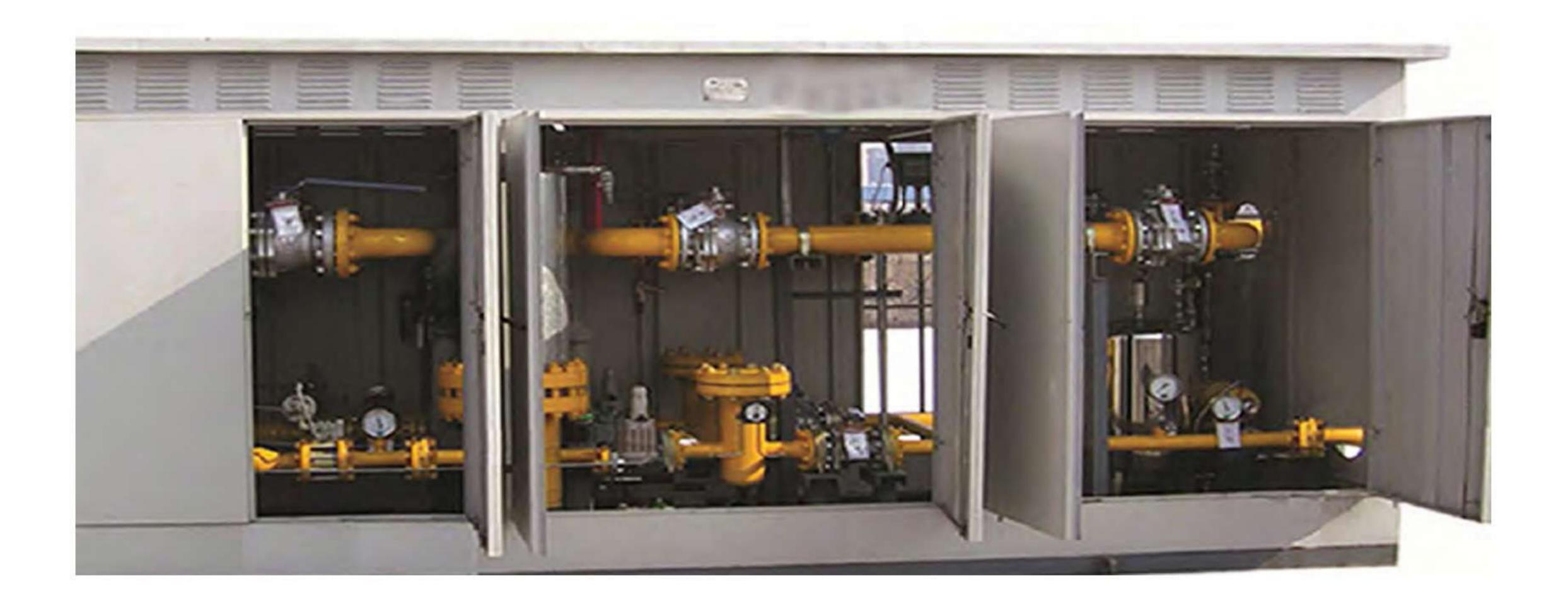
Skid-Mounted CNG Pressure Reducing Station is a set of Pressure Regulating and Metering Equipment, which makes the Compressed Natural Gas's pressure reduce to Pipeline's operating pressure by 2:3 step regulating. heat-exchange, metering and odorization, shipped by CNG tank car. The equipment has the characteristics of high-accuracy, compact structure, convenient maintenance, etc.
