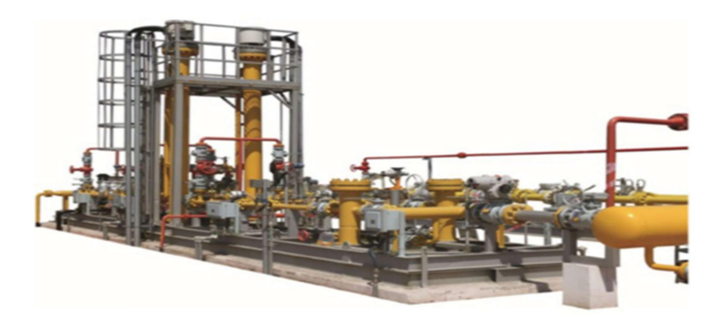
Gas metering and regulating system for gas turbine is a skid-mounted gas supply equipment for gas turbine in the compressor station of long distance gas pipeline, the system integrates the functions of filtering, heating, regulating, metering, venting, relief, leak alarm and automatic switching, having the characteristics of high explosion proof requirement, wide regulation range good safety performance and continuous stable gas supply.
