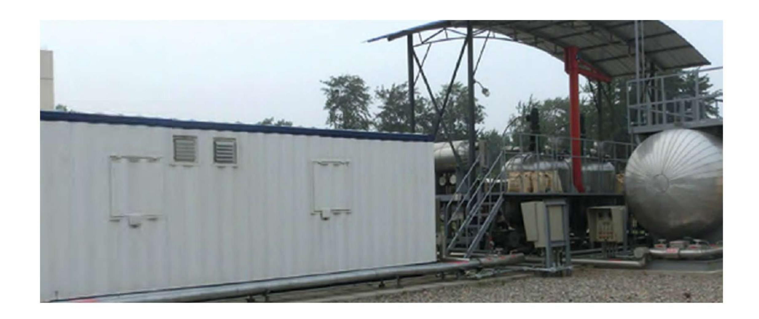
The main function of Injection System is mixing the material with crude oil, stirring the material to be melted and homogenized and then injecting the material to crude oil pipeline for depressing effect. The equipment applies the modular structure design, which has several characteristics, such as simple structure, safe and reliable system, high heating efficiency and fast operation.
