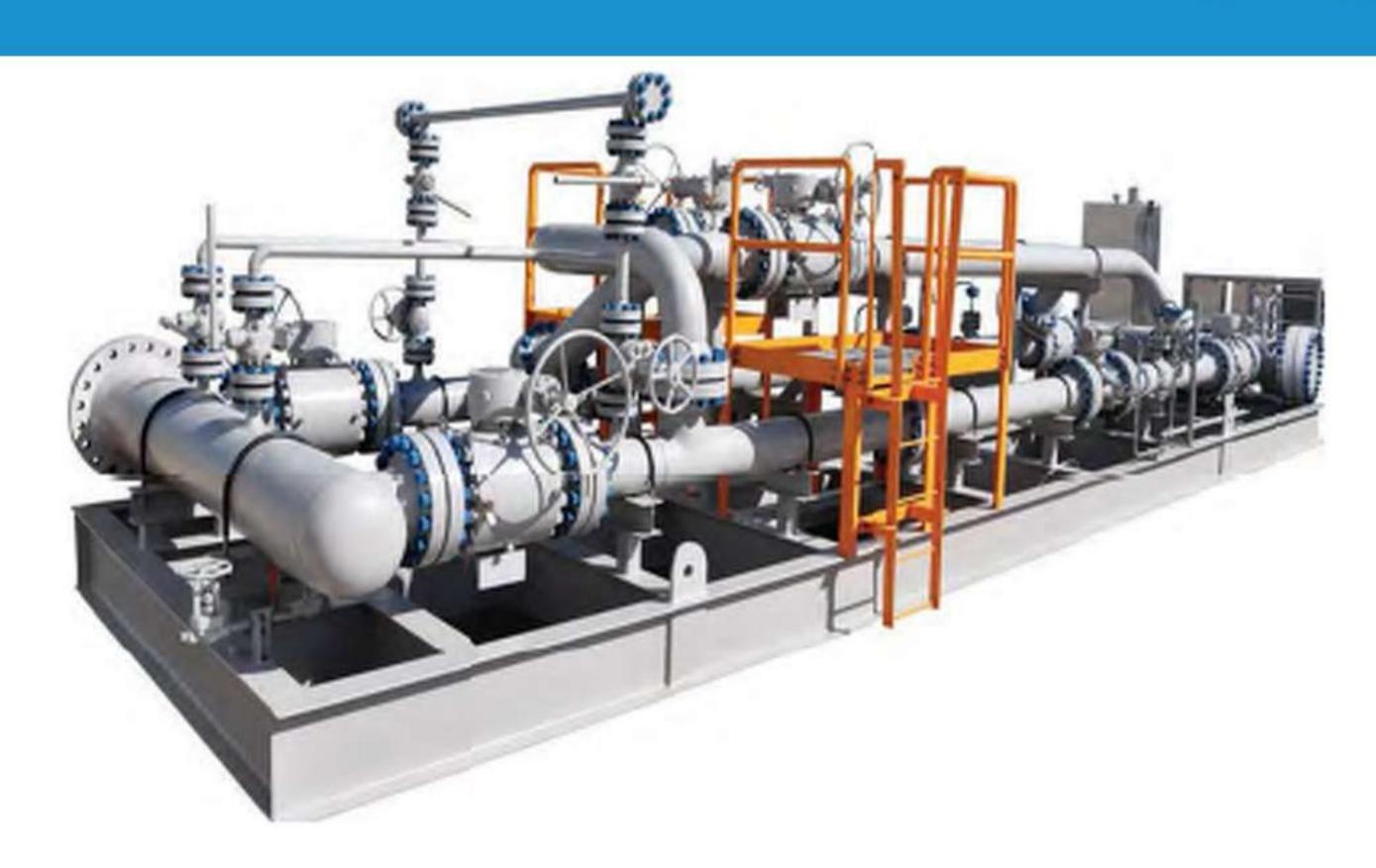
Turbine/ultrasonic metering system is a skid-mounted metering system for custody transfer metering in the metering station of long distance gas pipeline. The system integrates the functions of filtering (or the filtering part is separated), metering, flow ratios, on-line calibration, system venting, leak alarm and automatic switching, having the characteristics of high metering accuracy, good safety performance, continuous stable metering and high explosion proof requirement.
