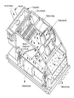
The mud flow should be spread over as much of the screen surface as possible by using feed-control gates located between the possum belly (flow line-to shaker transitional reservoir and the screen surface. The mud should cover 75% of the screens (About 1 foot from the end of the screens)
